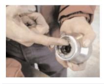
5.) Put a light film of grease around the lip of the Grease Seal to keep it from tearing during installation. Wipe off the excess grease prior to installing.
