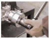
6.) Install the front Wheel Bearing and castle nut, torque the castle nut to 15 ft. lbs to seat the Wheel Bearings properly. Then loosen the castle nut to finger tight and rotate the Hub Assembly the hub should rotate freely. Line up the hole for the cotter pin through the castle nut by tightening the castle nut then double check that the Hub Assembly rotates freely and has no play on the Spindle.
