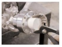
1.) Begin by removing the dust cap, using Channel Locks grasp the dust cap firmly and work up and down while pulling outward as well. Remove the cotter pin and castle nut set aside the castle nut and dust cap. Throw away the cotter pin, it will not be reused.
