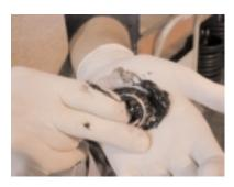
3.) Pack Wheel Bearings with Wheel Bearing Grease either by hand or with Wheel Bearing packing tool, forcing grease into the cage and roller assembly. Put a film of grease on both Wheel Bearing Races and on the Spindle shaft.
